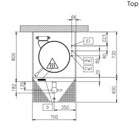
**Electric** 400 V/3N ph/50/60 Hz Supply voltage: Total Watts: 12.4 kW Installation:
